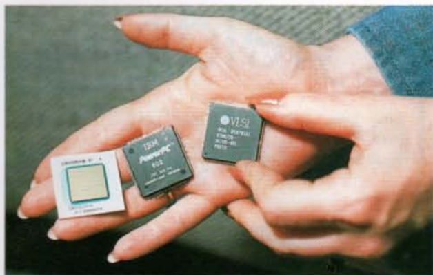
Left: the first M2 silicon includes (left to right) the graphics ASIC, the PowerPC 602 and a CD controller chip. Goldstar has produced this M2 mock-up (above)
